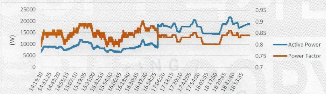
<Fig. 2> Variation curve of active power and power factor in overall test.
